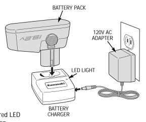
3. When fully charged, reattach battery pack onto Cordless Worklight, making certain latches fasten securely. Cordless Worklight will not operate properly if the battery pack is not seated properly.
